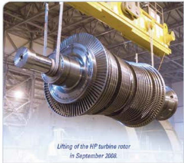
The HP turbine is a double-flow turbine consisting of inner and outer casing structures split horizontally.
