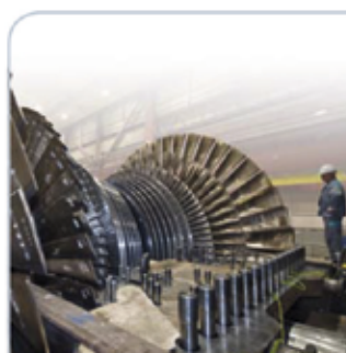
The OL3 LP turbines are double-flow turbines with running blades attached to blade wheel discs shrunk on to the turbine shaft.
