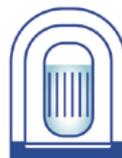
Double concrete walls of the gas-tight containment
