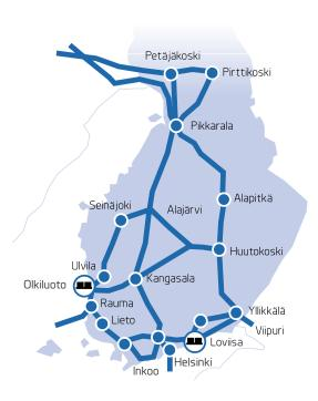
The Finnish electricity system consists of power plants, national and regional distribution grids as well as electricity consumers. Olkiluoto nuclear power plant is connected with the national grid of Fingrid Oyj by six 400 kV power lines and two 110 kV lines. The 110 kV lines go to the power station in Rauma and the 400 kV lines to Ulvila (2 lines), Huittinen, Kangasala and Rauma (2 lines).
