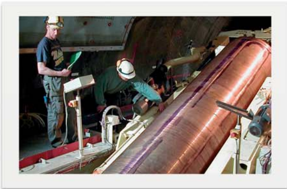
Canister emplacement test in Äspö hard rock laboratory in Sweden.
