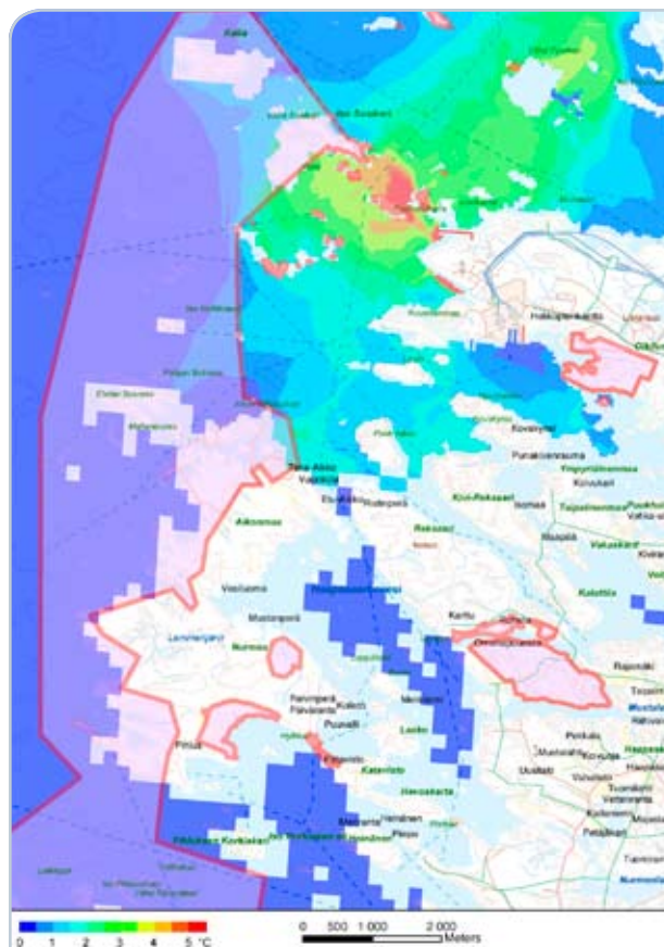
Figure 9-47 Limits of the Rauma archipelago Natura 2000 area and the spreading of cooling water at a depth of 2.5 metres during a south wind, cooling water intake at point C and discharge at point B.
