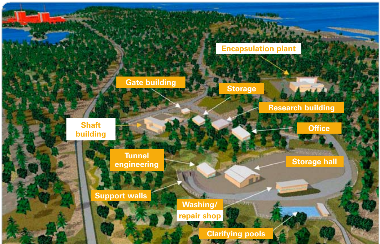
Figure 9-5 Visualisation of the parts of the final disposal facility located above ground (Posiva).
