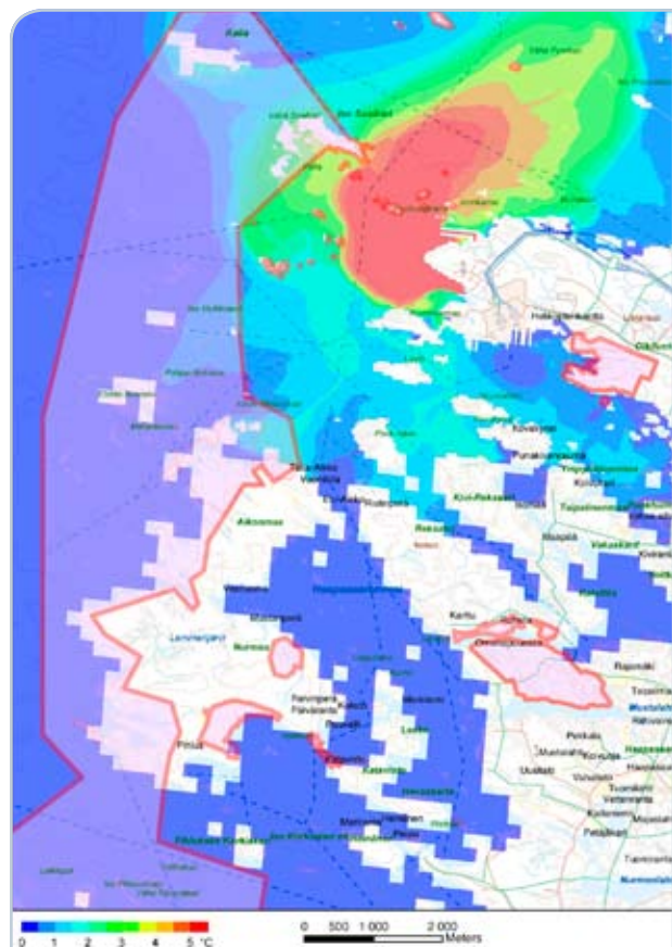
Figure 9-46 Limits of the Rauma archipelago Natura 2000 area and the spreading of cooling water in surface water during a south wind, cooling water intake at point C and discharge at point B.
