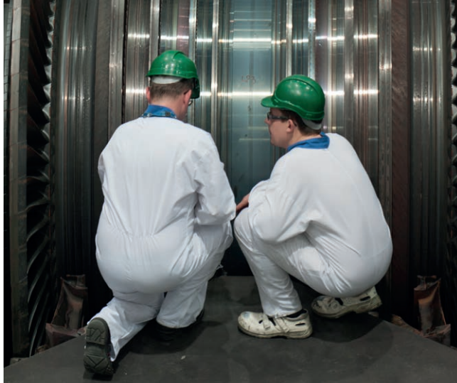
Inspection of the clearance between the rotor and stator vanes on low pressure turbines.
