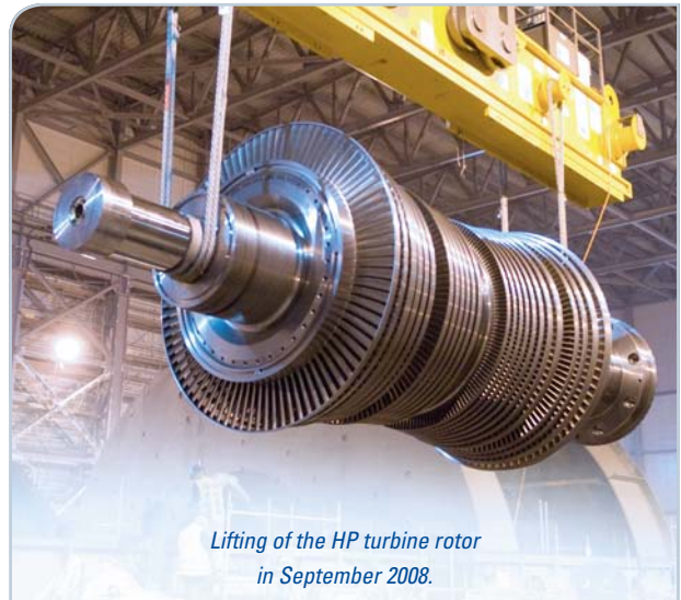
The HP turbine is a double-flow turbine consisting of inner and outer casing structures split horizontally.
