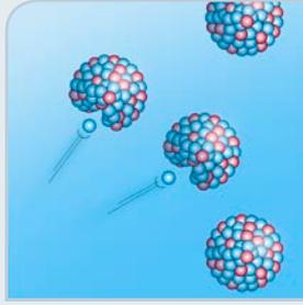
The moderator at OL3 is water. Moderation reduces the speed of a neutron to 4.4 km/s, thus its potential to split uranium nuclei is increased.
