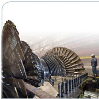
*The turbines in OL3 have the highest electric output in the world. The diameter of one low-pressure turbine is almost seven metres at its widest.*
