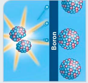
At OL3, the fission and the power of the reactor are controlled by adjusting the control assemblies and regulating the boron content in the coolant water.
