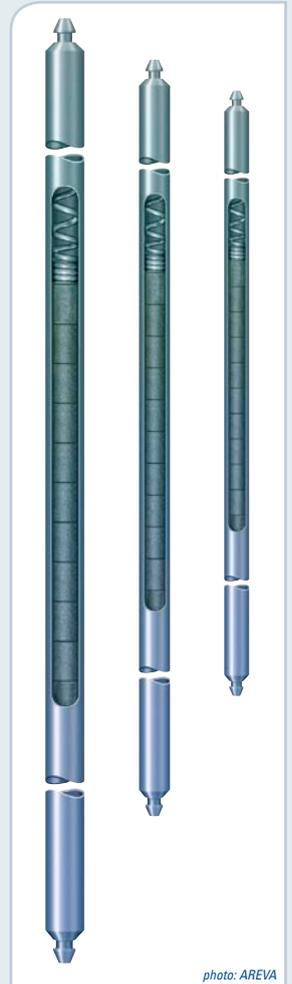
>> One fuel assembly contains 24 guide thimbles and 265 fuel rods (pictured). One fuel rod contains hundreds of fuel pellets. The metallic cladding of the fuel rod is the first barrier between the environment and the radioactive substances developing in the fuel.
