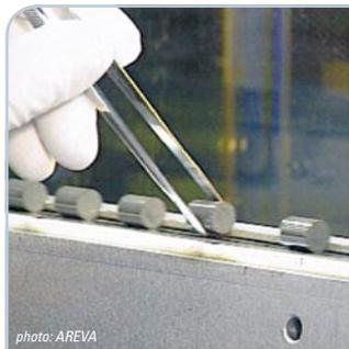
*One fuel rod contains hundreds of fuel pellets. Approximately eight fuel pellets is enough to produce electricity for one year for a family of four living in a detached house with direct electric heating.*
