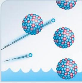
Neutrons move at a speed of about 20,000 km/s. Without a moderator, the speed of these so-called fast-moving neutrons is so high that uranium atoms cannot absorb them, which means that no remarkable extent of fission takes place.
