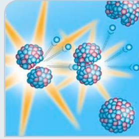
In fission, two new atoms and two or three fast-moving neutrons are created. These are moderated by water and can, in turn, split more uranium atoms, maintaining the chain reaction.
