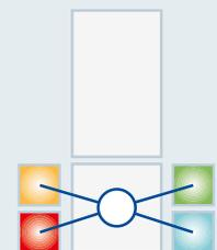
*The parallel subsystems of various safety systems are located in such a manner that any simultaneous failure of them by fire or for other reasons is unlikely.*
