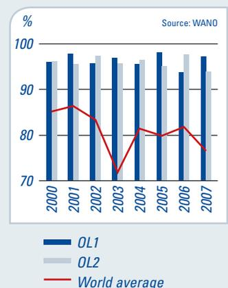
*The capacity factor is the share of electricity produced over a certain period of time as a percentage of the electricity that the unit would have produced over that same period of time if it had operated without disturbances at full capacity.*
