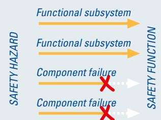
*Safety systems consist of several parallel and mutually redundant subsystems.*
