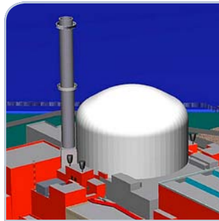
Offgases are delayed, filtered and conveyed from the plant into the atmosphere through a 100-metre-high ventilation stack.
