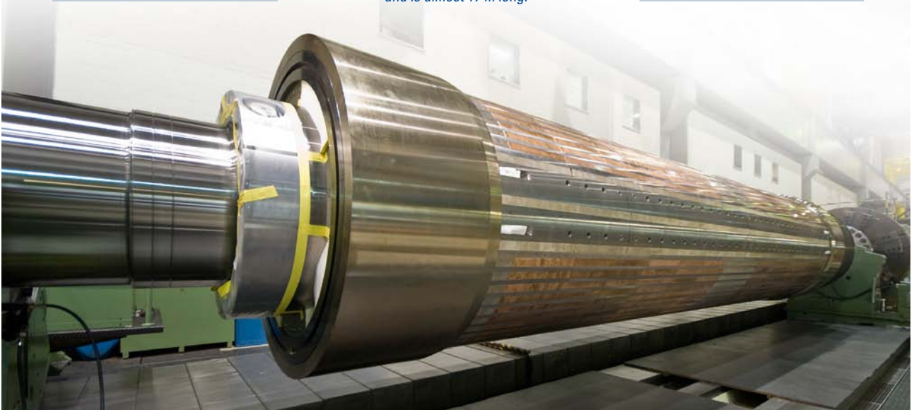
The hydrogen-cooled generator rotor rotates at 1,500 r.p.m., weighs 250 t and is almost 17 m long.
