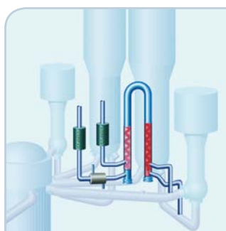
The boron content of the make-up water added to the primary circuit is monitored with double continuous-action measurement devices that control the automatic safety function.
