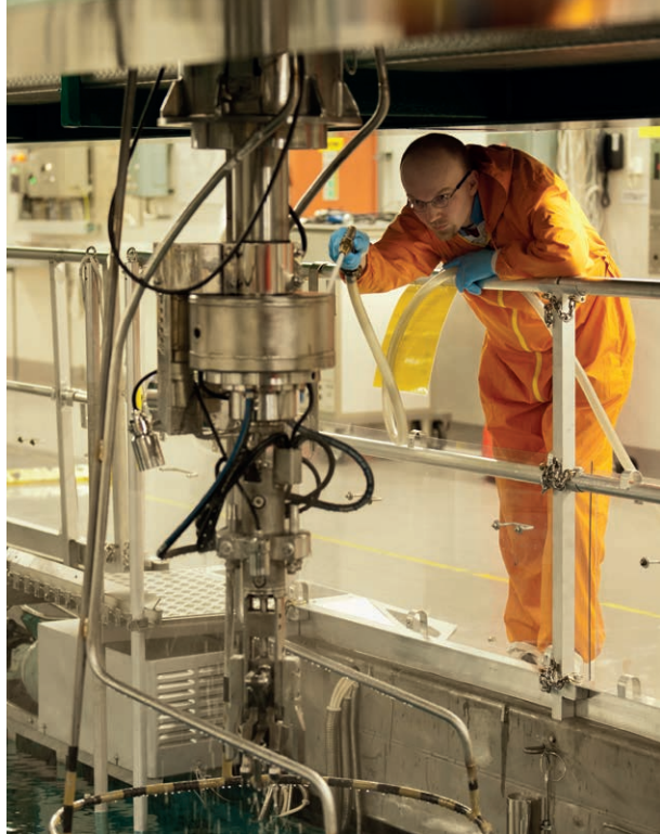
During the outages, Jussi Leino from RTK-Palvelu Oy is also responsible for rinsing the grapple hook on the refuelling machine.
