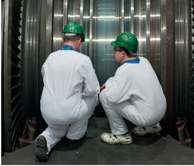
Inspection of the clearance between the rotor and stator vanes on low pressure turbines.
