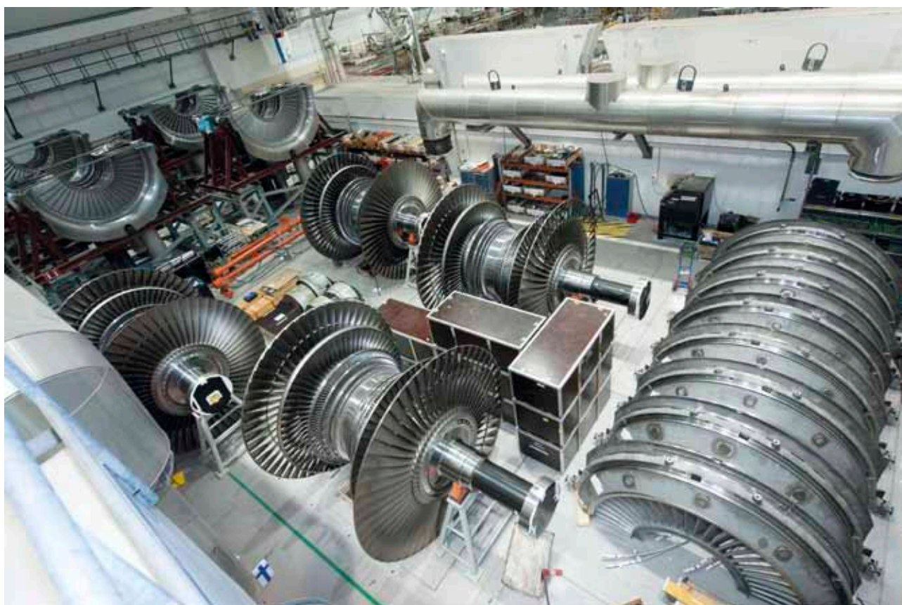
The OL1 and OL2 turbine plants were modernized in the course of the annual outages of 2010–2012. The modernization included, for example, the replacement of the LP turbines and the generators.
