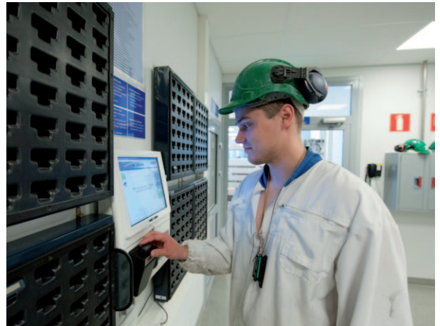
An electronic work dosimeter system is used to monitor personal radiation doses in real time.
