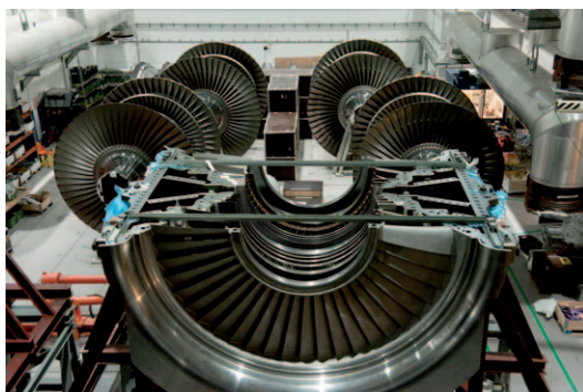
In the foreground, a low pressure turbine case; in the background, rotors.
