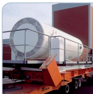
Spent fuel assemblies are transported to the interim storage facility in a transfer container made of spheroidal graphite cast iron.
