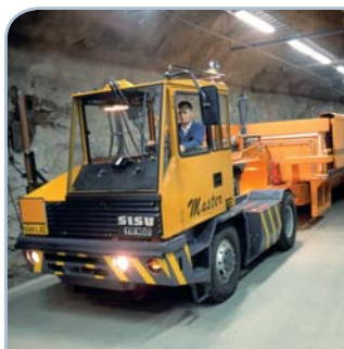
Waste is taken to the repository with a radiation-shielded vehicle.
