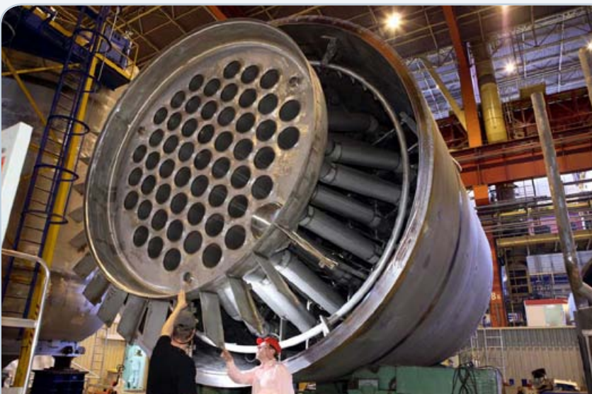
Internal parts of the secondary side of the steam generator being installed at the factor in France.
