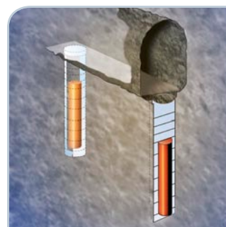
Construction of the final repository is preceded by careful studies of the integrity and geological stability of the bedrock. The spent fuel will be packed in copper-cast iron canisters and stored some 420 m below ground.
