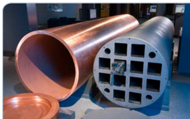
Figure 9-7 The final disposal canister consists of a copper jacket and an inner core made of nodular graphite cast iron. The final disposal canister can accommodate 12 spent fuel bundles used in OL1 and OL2 as illustrated, or four fuel bundles of an EPR of the OL3 type.
